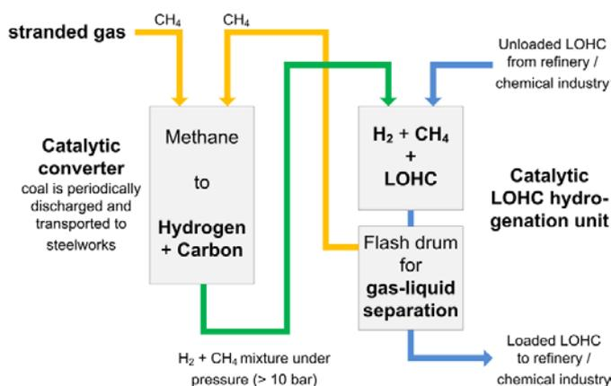
Figure 1: Two-step upgrading process for stranded gas
